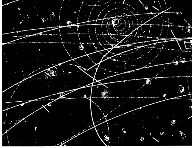
Figure 4.5 Example of the reaction K^- + p \rightarrow \Lambda + \pi^0 occurring when a K^- -meson comes to rest in a hydrogen bubble chamber, at the point A . The neutral pion undergoes Dalitz decay, \pi^0 \rightarrow e^+ e^- \gamma . The \Lambda -hyperon decays ( \Lambda \rightarrow \pi^- + p ) at the point B . (Courtesy CERN.)
