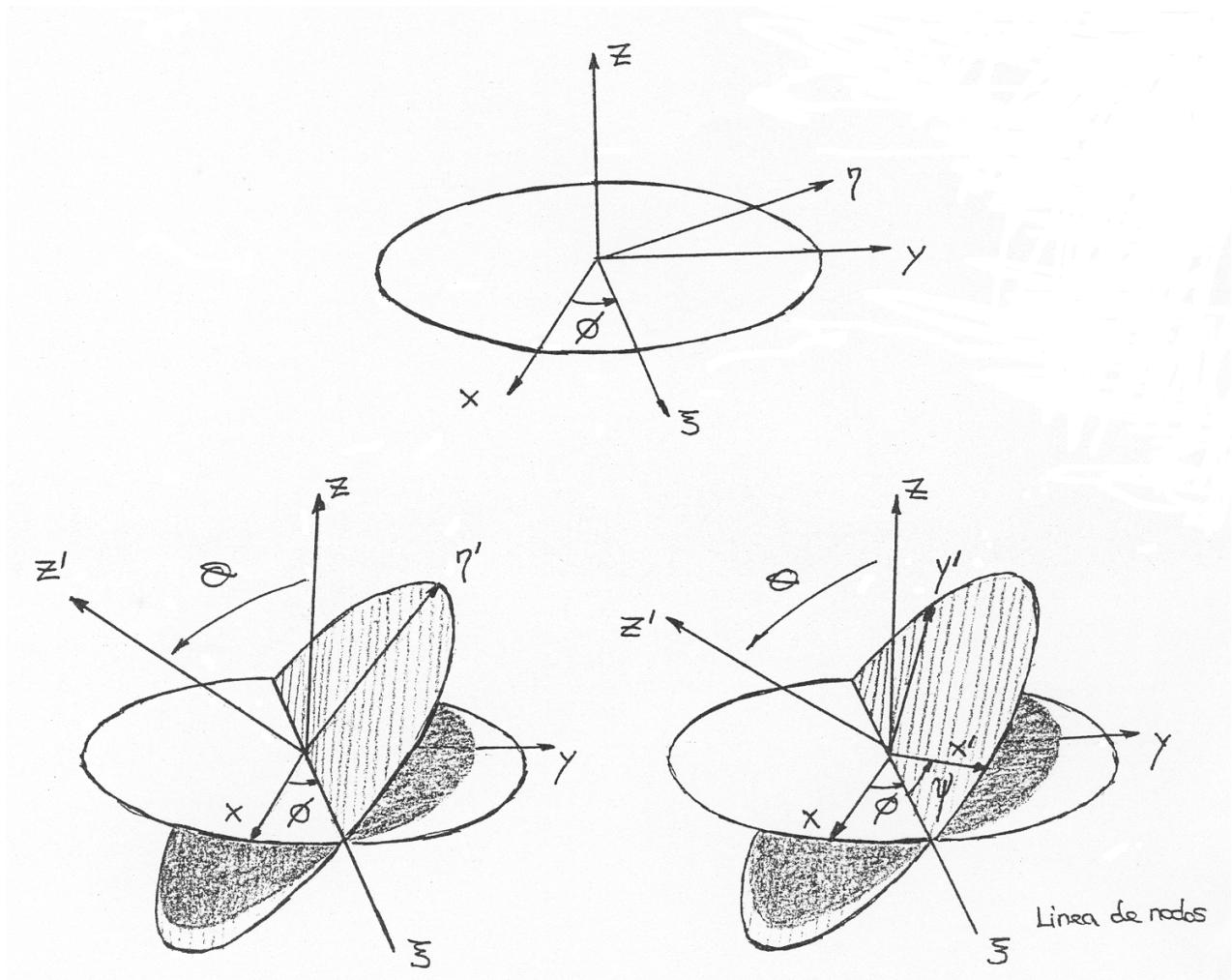
$$A = \begin{pmatrix} \cos \phi \cos \psi - \sin \phi \cos \theta \sin \psi & \sin \phi \cos \psi + \cos \phi \cos \theta \sin \psi & \sin \theta \sin \psi \\ -\cos \phi \sin \psi - \sin \phi \cos \theta \cos \psi & -\sin \phi \sin \psi + \cos \phi \cos \theta \cos \psi & \sin \theta \cos \psi \\ \sin \phi \sin \theta & -\cos \phi \sin \theta & \cos \theta \end{pmatrix}$$
